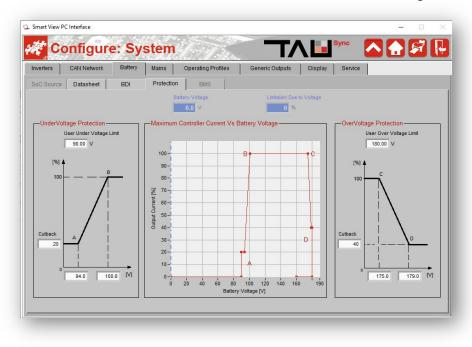
Figure 6 - Battery Protection
