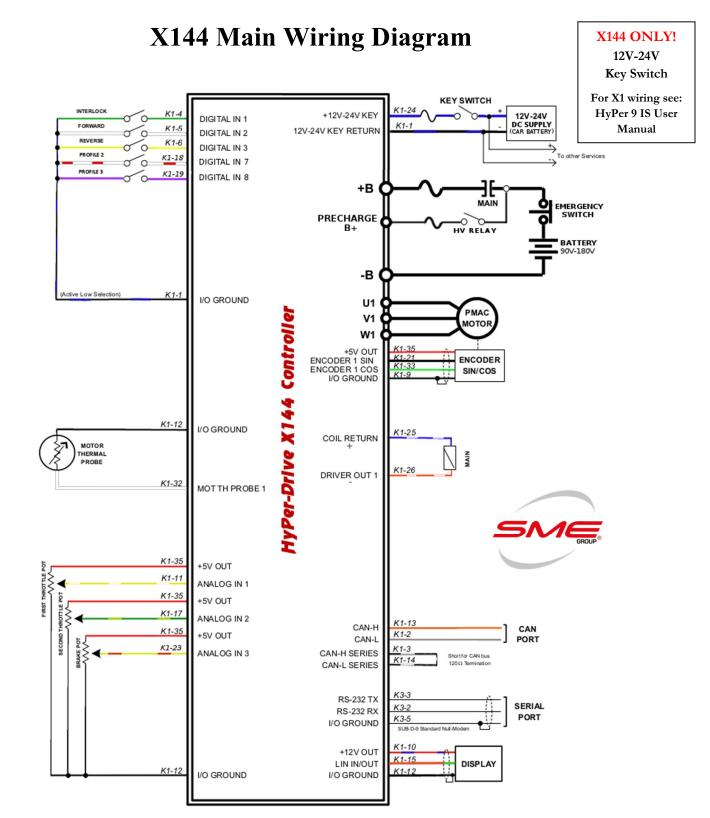
Figure 2 - Standard X144 Wiring Diagram
