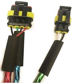
Figure 4 - Motor Plug Wiring Photo
